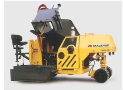
Hydraulic Tilting Inlet Chute
