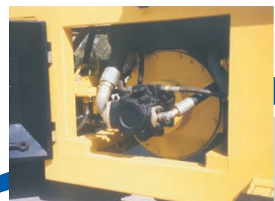
Main Hydraulic Pump
