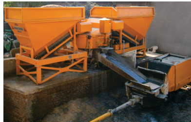
Mixed Concrete discharged directly in to the Concrete Pump
