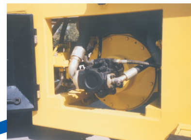
Main Hydraulic Pump
